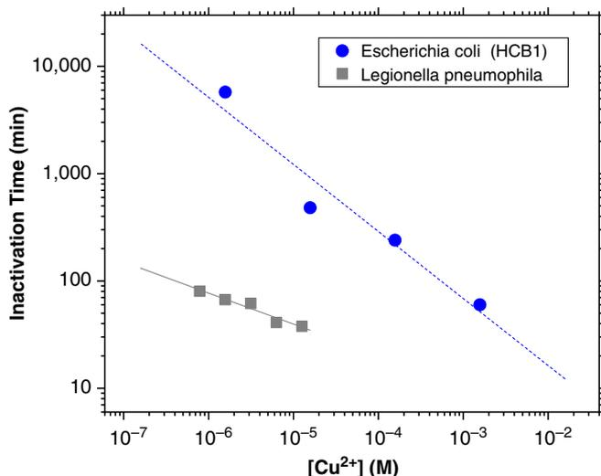
**FIGURE 2.** Inactivation time (>99.9% reduction) of *Escherichia coli* (HCB1) and *Legionella pneumophila* bacteria in various soluble [Cu<sup>2+</sup>] concentrations. Data from Foster, et al.,<sup>32</sup> and Lin, et al.<sup>33</sup> Trend line indicates a regression fit.
